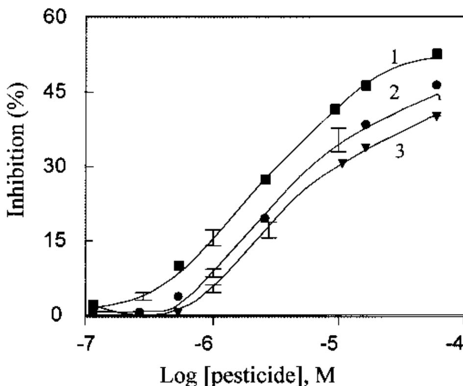
**Figure 5.** Determination of pesticides with the amperometric AChE-PB modified sensor (0.1M phosphate buffer, pH 7.2, containing 0.05M KCl and 0.1 mM AChE, at 25°C). 1-Dichlorvos; 2- Diazinon; 3-Fenthion.
