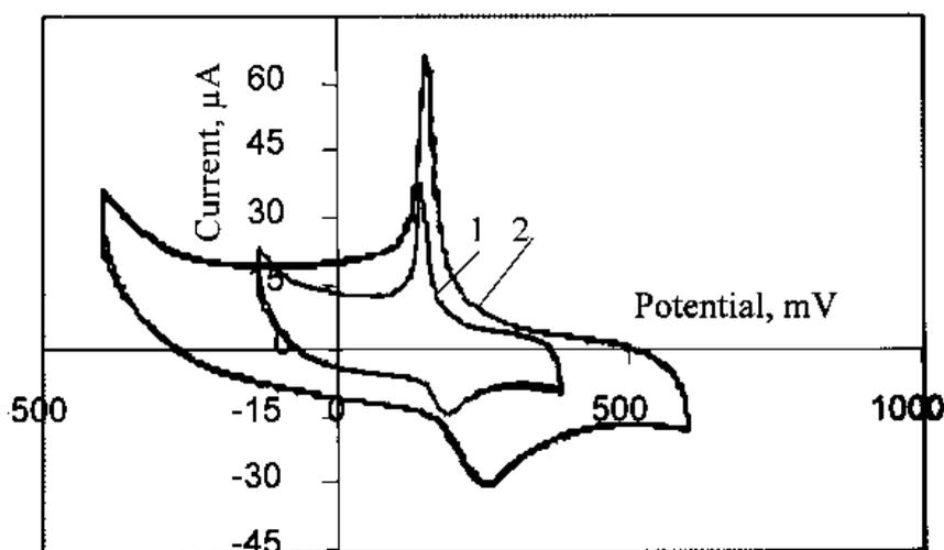
**Figure 2.** Cyclic voltammograms of (1) PB and (2) PEI-PB modified graphite electrodes in 0.5M KCl solution, 300 rpm, 20<sup>o</sup> C.
