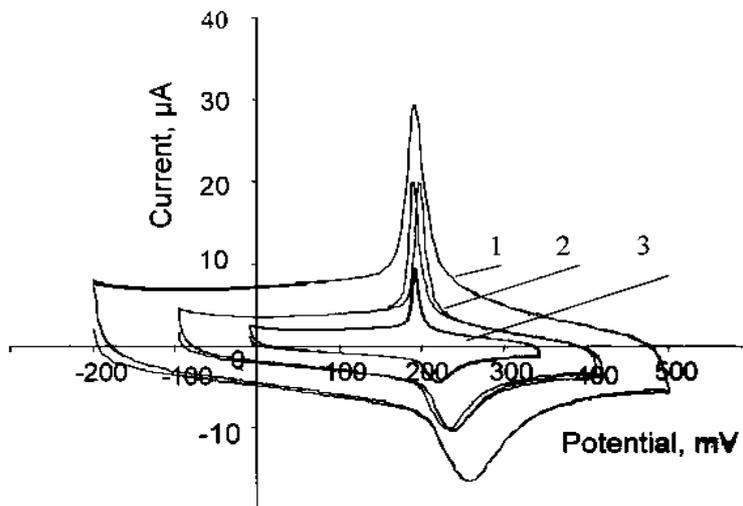
**Figure 1.** Cyclic voltammograms of Prussian Blue modified carbon electrode in a 1.0M KCl solution, pH 5.0, at different scan rates. Scan rates: (1) 100 mV/s; (2) 50 mV/s; (3) 20 mV/s.
