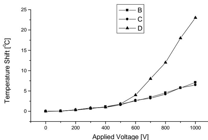
**Figure 1.** Temperature shift vs applied voltage. B - theoretical assumption, C - measured temperature for non ionic buffer, D- measured temperature for PBS buffer. All records are for exponential pulses.
