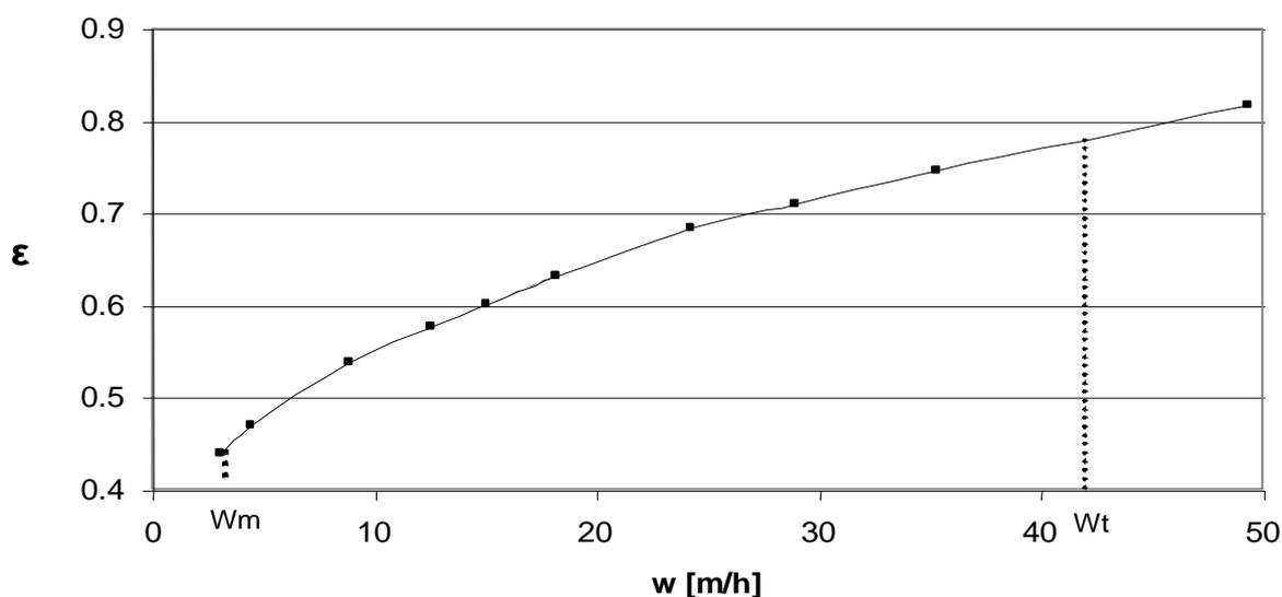
For a  $30 \text{ m h}^{-1}$  value of the superficial velocity in the column, the fluidized bed porosity was 0.72. Specific surface, in the fluidized bed with a void fraction of 0.72, was calculated [2] with the formulae  $\sigma = 6(1-\varepsilon) \psi^{-1} \bar{d}^{-1}$ , resulted a value of about  $7000 \text{ m}^2 \text{ m}^{-3}$ . With the dimensions of working fluidized bed, a value of about  $20 \text{ m}^2$  available for biofilm growth is obtained.
