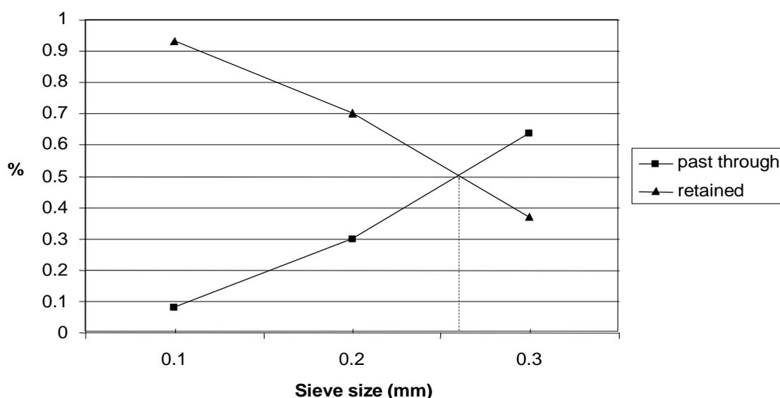
A mean value for the particle diameter of 0.26 mm resulted. Shape factor for support particles, calculated [4] with the formulae  $\varepsilon_0 = (0.083 \psi)^{1/3}$  where  $\varepsilon_0 = 0.43$  is the void fraction of unexpanded bed resulted in a value of  $\psi = 0.95$ .
