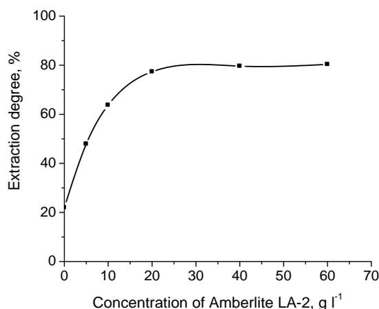
**Figure 2.** Influence of extractant concentration of reactive extraction yield (extraction duration = 60 s).
