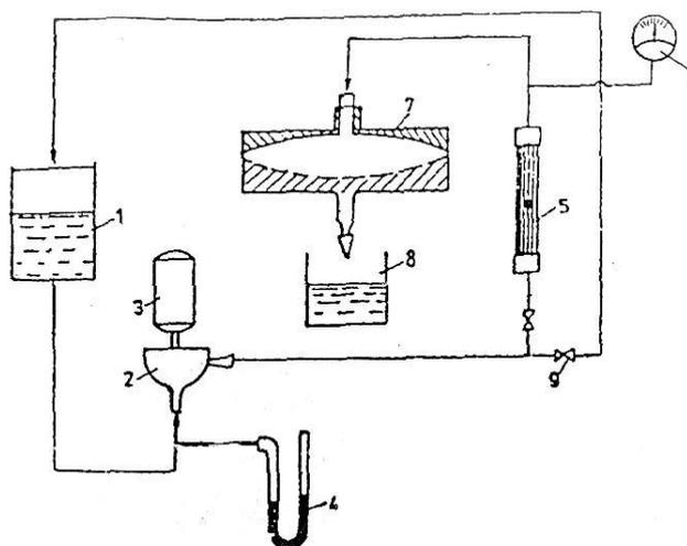
**Figure 1.** The UF-MF laboratory installation
