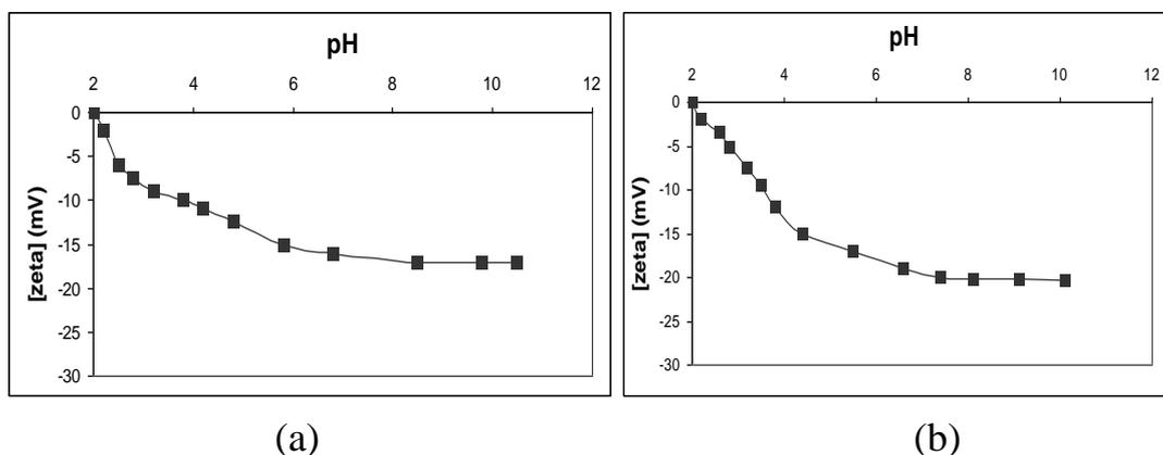
Figure 5. [zeta] potential/pH profile for (a) MB<sub>2</sub> polyurethane membrane and (b) MB<sub>1</sub> polyurethane membrane
