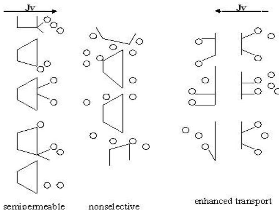
**Figure 3.** Differences in transport properties between usual semi-permeable membranes and a charge membrane
