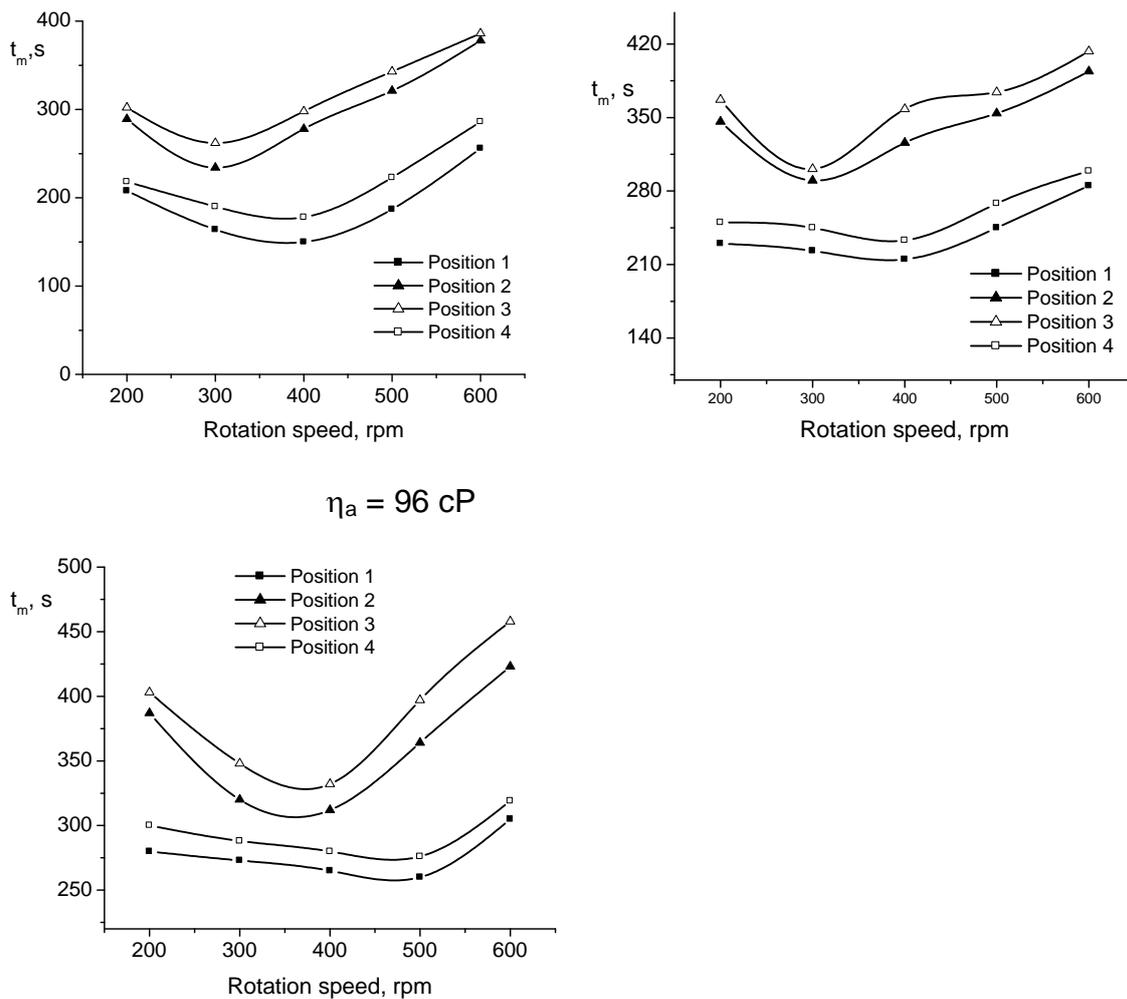
**Figure 1.** Influence of rotation speed on mixing time (aeration rate of  $75 \text{ l h}^{-1}$ ).
