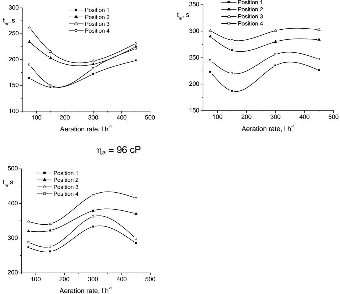
**Figure 3.** Influence of aeration rate on mixing time (rotation speed 300 rpm).
