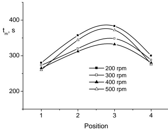
**Figure 2.** Influence of pH electrode position on mixing time (aeration rate of 75 l h<sup>-1</sup>).
