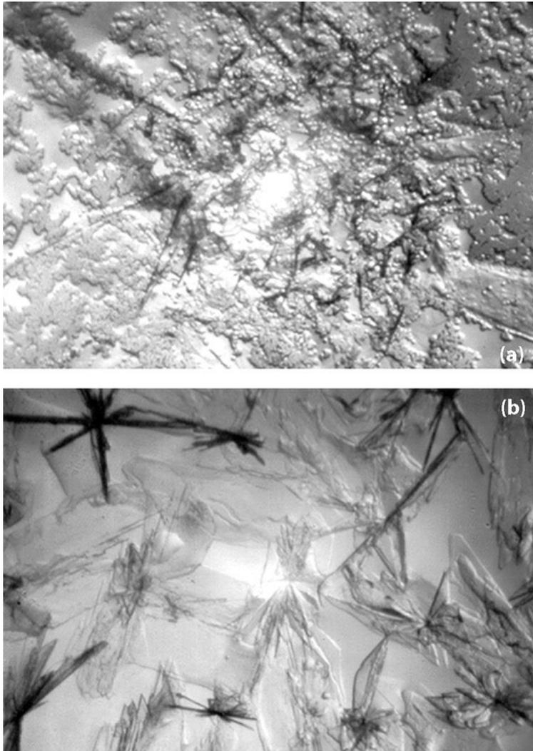
Fig. 15 – Crystals grown by means of technique 2 in absence (a) and in presence of 0.022 µg/ml (b) OPN which slowed the kinetic of the brushite → OCP phase change. (a) and (b) 20X. Note that OPN prevented the growth of OCP spherulites clearly visible in (a) and it caused the lost of the original habitus of the brushite crystals and the increase in the surface area of their {010}'s (b).
