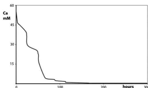
Fig. 3 – Reduction of the calcium concentration of the calcium phosphate reacting solution used for crystal growth technique 2 at 21 °C. To plot this curve were utilized the solutions of 24 crystallization baths since the experiments were broken off after fixed times.
