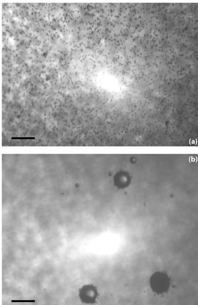
Fig. 14 – Spherulites of HAP grown by means of technique 2 respectively in presence of  $4 \times 10^{-4}$   $\mu\text{g/ml}$  (a) and  $0.04 \mu\text{g/ml}$  (b) OPN. Notice the increase in size of the hemispheric aggregates grown in presence of  $0.04 \mu\text{g/ml}$  OPN. Bar  $300 \mu\text{m}$ .
