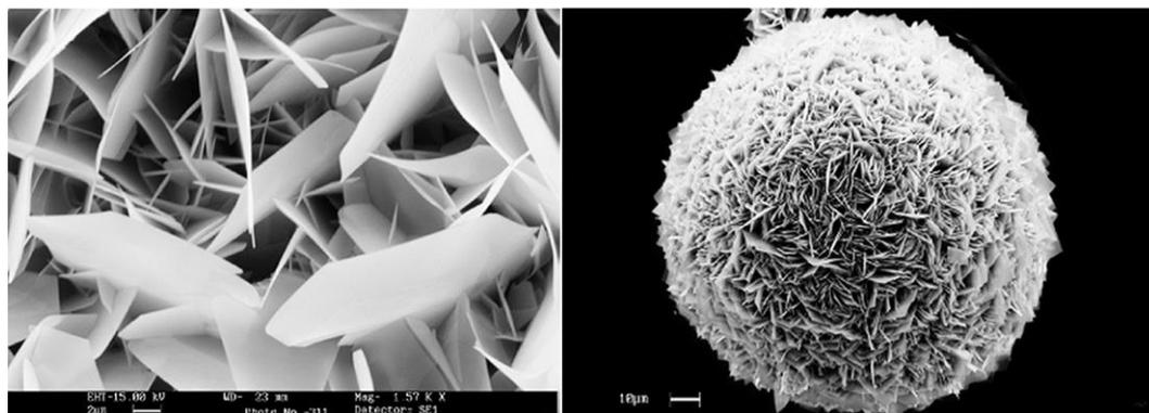
Fig. 8 – Scanning electron micrograph: OCP prismatic hexagonal single crystals (size apparent values 10 x 5 x 0.6  $\mu\text{m}$ ) aggregated to form spherulites.
