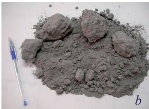
Fig. 1 – a) Extractive front of the “Il Calvario” quarry, where the vertical fractures present superficial mineralization of prismatic yellow fluoro-edenite amphibole; b) fine grained volcanic material of the “autoclastic breccia” (fractured and crumbled benmoreite lava) containing the fluorine fibrous amphiboles.
