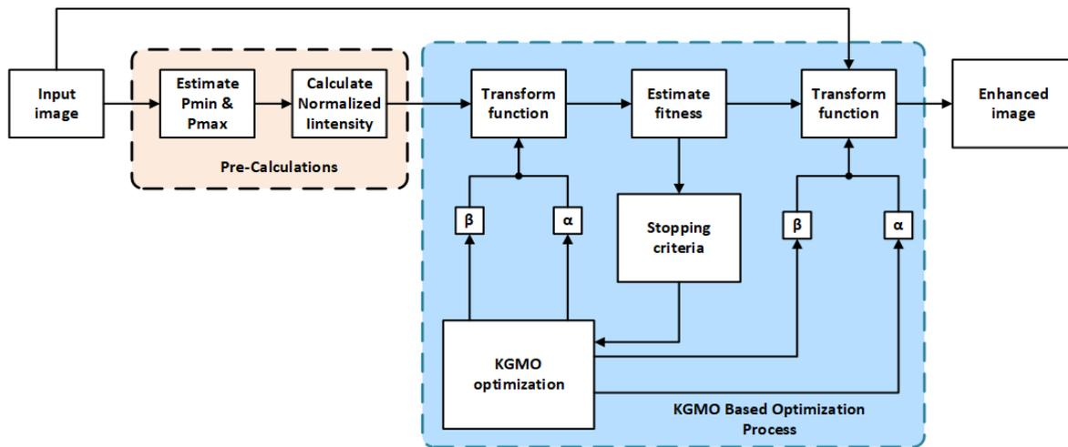
Figure 2. Block diagram KGMO optimization process
