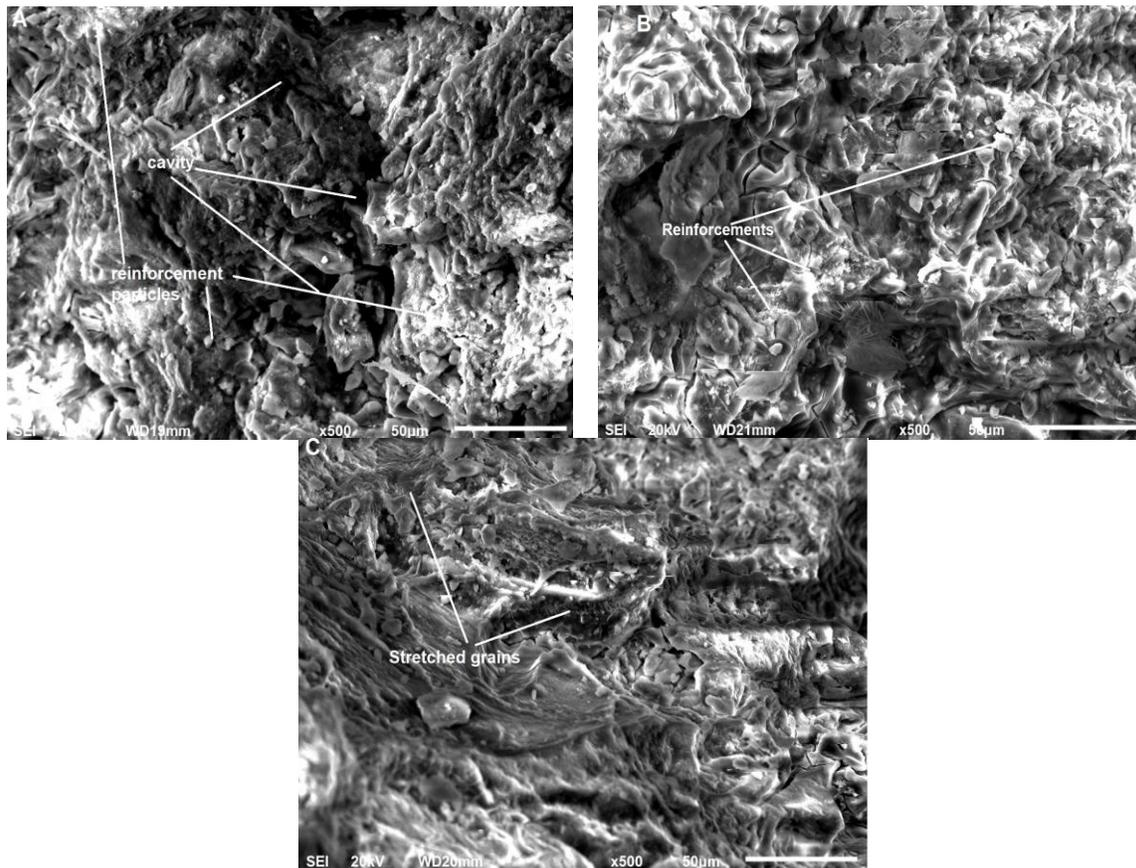
Fig.2 SEM of Mg composite (A) as-extruded Mg- composite with 2% Al<sub>2</sub>O<sub>3</sub> (B) heat treated Mg-composite with 1% Al<sub>2</sub>O<sub>3</sub> (C) heat treated Mg-composite with 2% Al<sub>2</sub>O<sub>3</sub>
