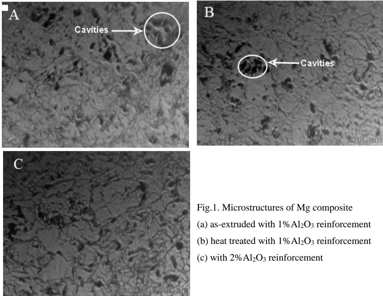
Fig.1. Microstructures of Mg composite
