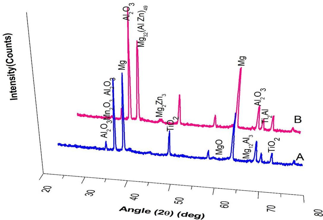
Fig. 3. X-ray diffraction of heat treated Mg-composites (A) 1% Al<sub>2</sub>O<sub>3</sub> and (B) 2% Al<sub>2</sub>O<sub>3</sub>
