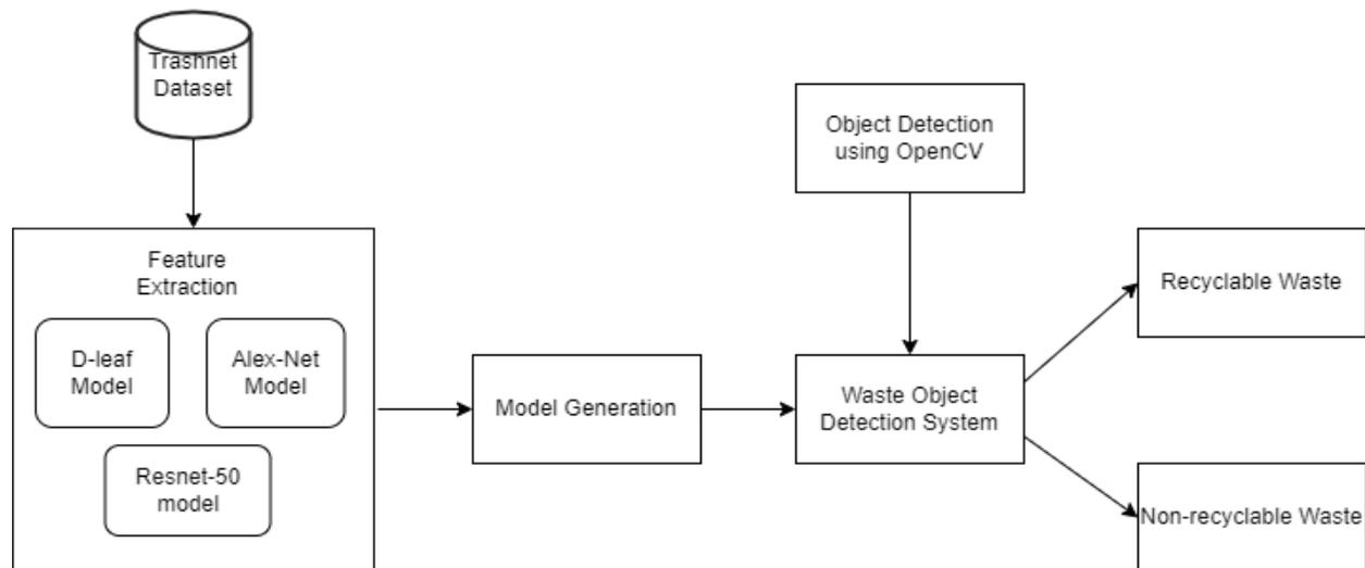
*Figure 2 System design for waste classification*
