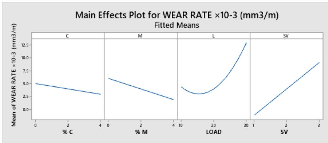
Figure 2. Main Effects Plot wear rate for AA7075/cenosphere/MoS<sub>2</sub> composites
