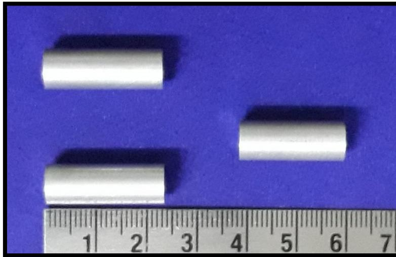
**Figure 1.** Photographic image of composite pins machined to the dimensions Ø8 mm × 22 mm
