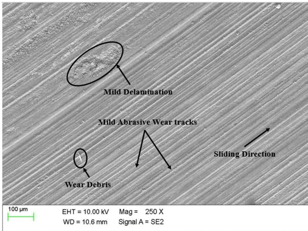
**Figure 5.** SEM image of worn surface for optimum condition 20 N applied load and 1 m/s for AA7075/cenosphere/MoS<sub>2</sub> composites
