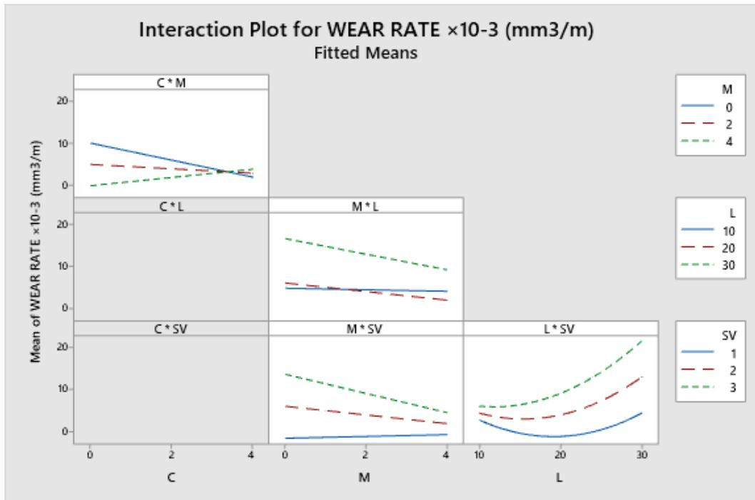
Figure 3. Interaction Plot wear rate for AA7075/cenosphere/MoS<sub>2</sub> composites
