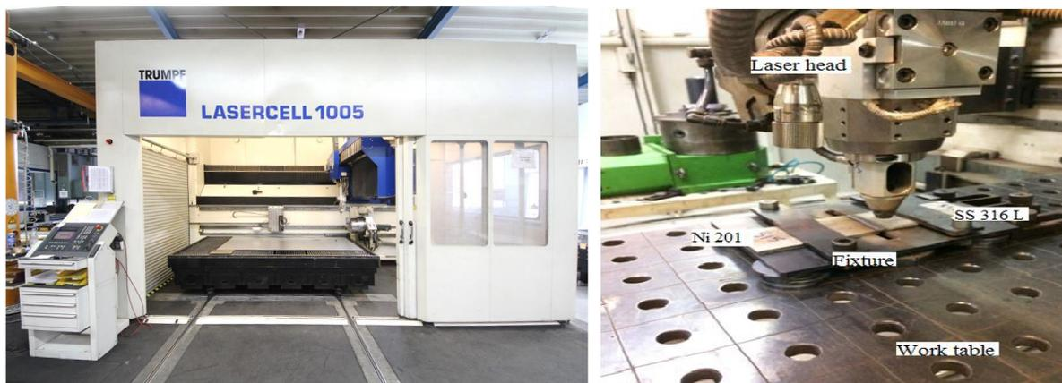
**Figure 1.** Experimental Setup of the TRUMPF LASERCELL TLC1005
