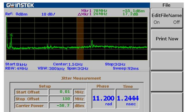
Fig.3.10. Phase Jitter of OCM signal with ADM modulation under cancerous tissue
