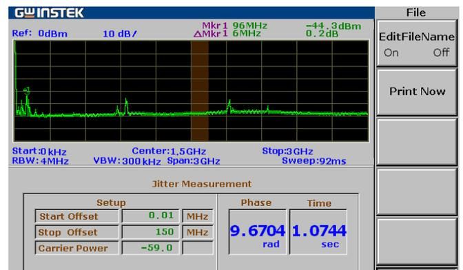
Fig.3.6 Phase Jitter of OCM signal with ASK modulation under cancerous tissue
