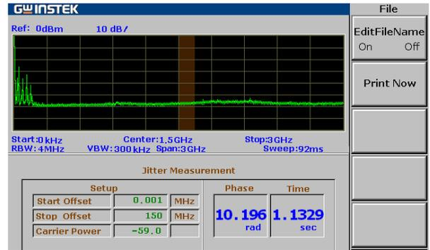
Fig. 3.2 Phase Jitter of OCM signal with PWM under cancerous tissue
