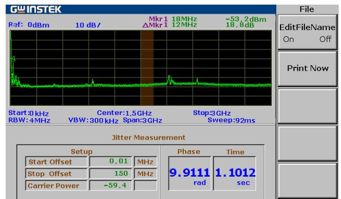
Fig.3.12. Phase Jitter of OCM signal with PSK modulation under cancerous tissue
