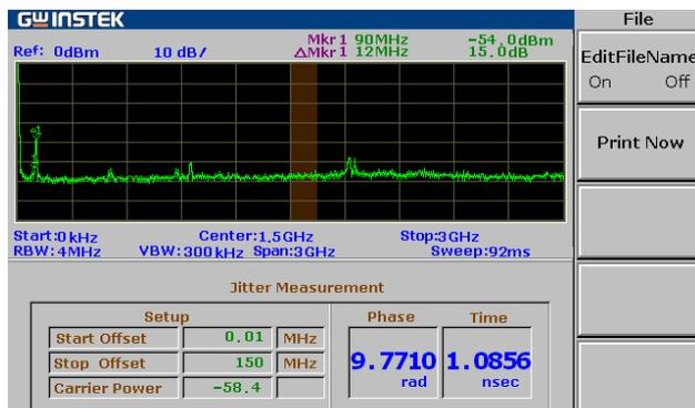
Fig.3.9. Phase Jitter of OCM signal with ADM under normal tissue
