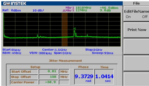
Fig.3.12. Phase Jitter of OCM signal with PCM under normal tissue
