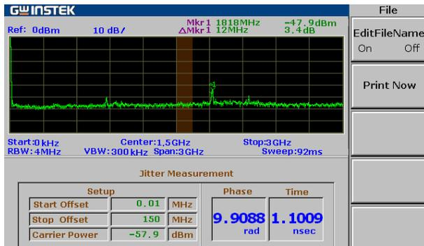
Fig. 3.7. Phase Jitter of OCM signal with QPSK modulation under normal tissue
