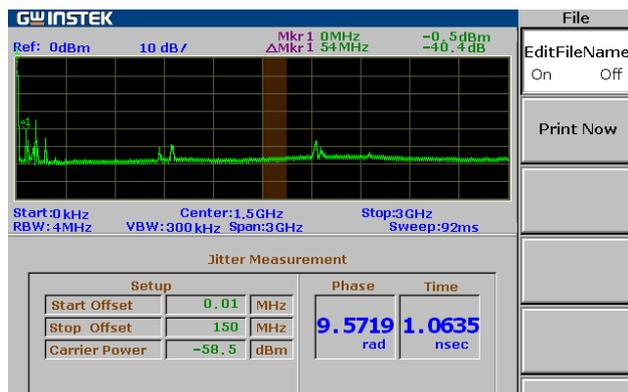
Fig. 3.5 Phase Jitter of OCM signal with ASK modulation under normal tissue
