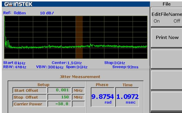
Fig. 3.1 Phase Jitter of OCM signal with PWM under normal tissue
