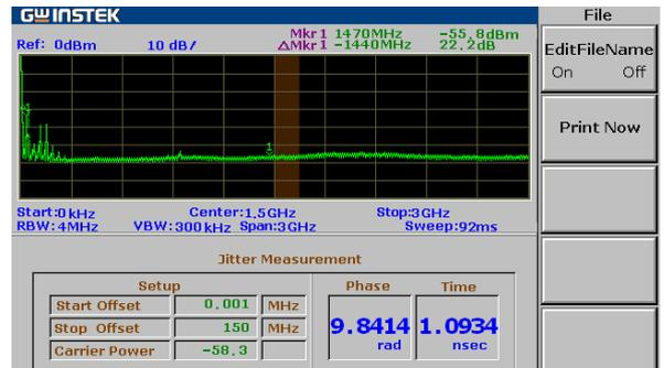
Fig.3.15. Phase Jitter of OCM signal with PPM under cancerous tissue
