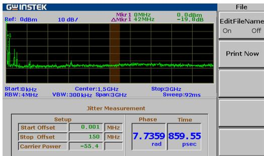
Fig.3.14. Phase Jitter of OCM signal with PPM under normal tissue
