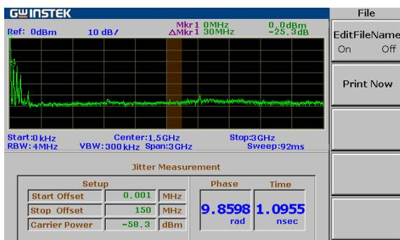
Fig. 3.3. Phase Jitter of OCM signal with PAM under normal tissue
