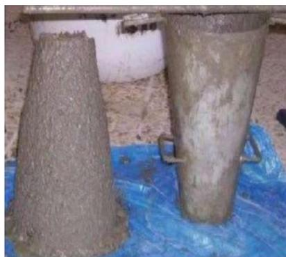
Fig. 5: Slump test result
