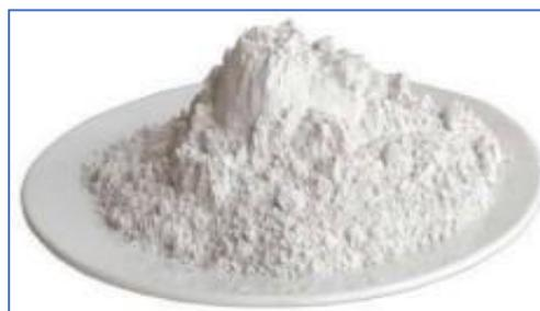
Fig. 3: Ground Granulated Blast Furnace Slag
