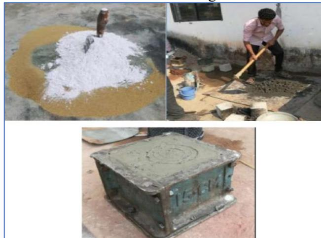
Fig.6: Preparation of concrete cube
