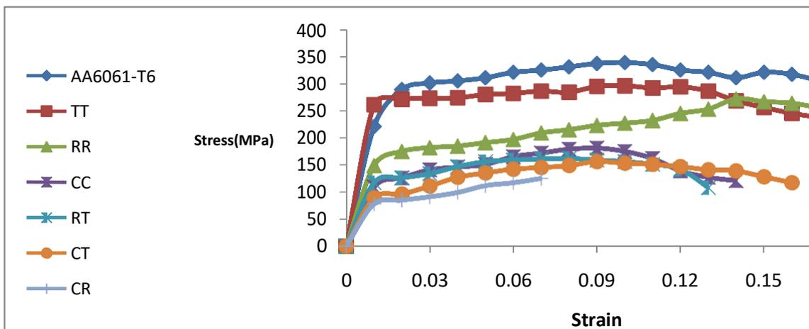
Fig 6. Stress–strain curves for FSW samples manufactured through the use of various dual-pin tools.
