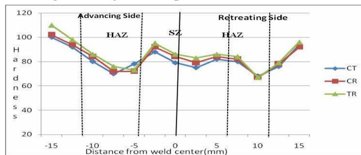
Fig 9. Micro-hardness distribution in the specimens fabricated by the tools with similar pins.
