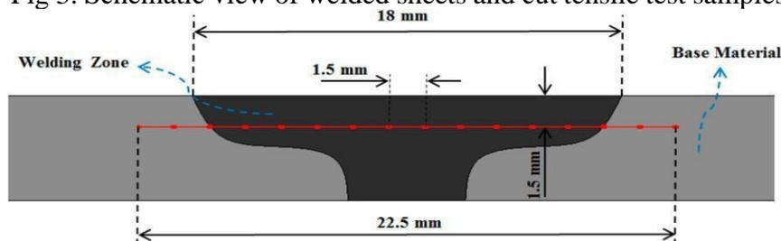
Fig 4. Schematic view of the locations of the hardness test measurements in the cross-sectional area of the joint sample.
