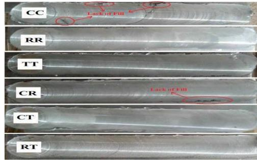
Fig 5. The top surface view of welded specimens with different dual-pin tools.
