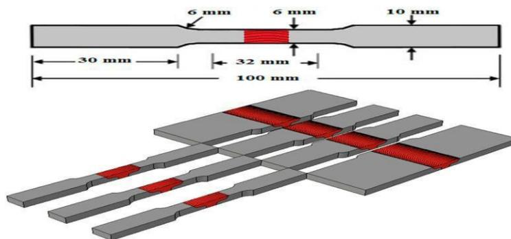
Fig 3. Schematic view of welded sheets and cut tensile test samples.
