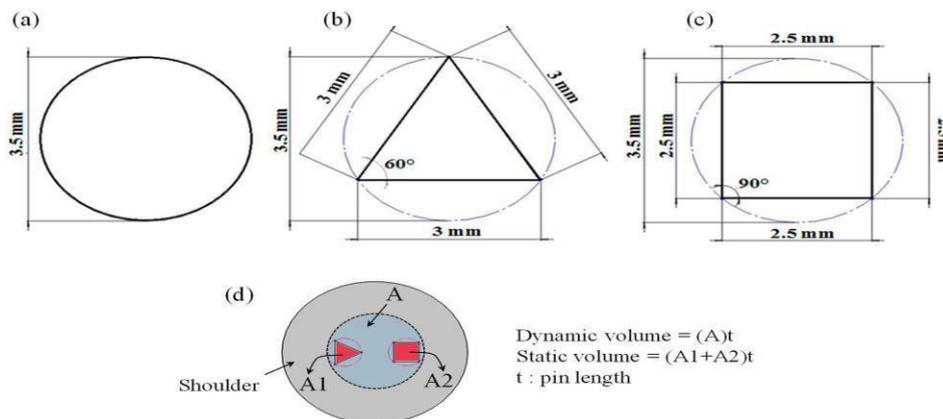
Fig 2. Geometric views and dimensions of (a) circular pin, (b) triangular pin, (c) square pin, and (d) terms used for a typical dual-pin tool.
