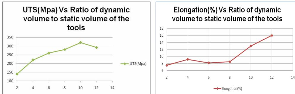
Fig 7. Values of UTS and elongations versus the ratio of dynamic volume to the static volume of the tools.
