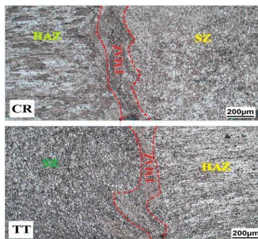
Fig 13. Microstructural features for different weld regions through CR and TT tools.
