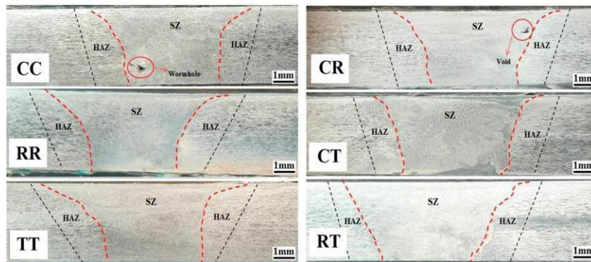
Figure 12. Macrographs of welded joints through the use of various dual-pin tools.
