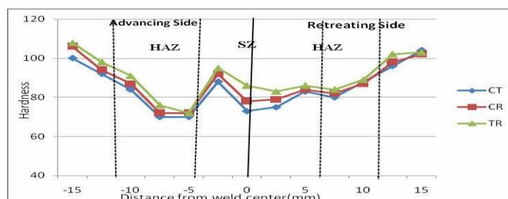
Fig 10. Micro-hardness distribution in the specimens fabricated by the tools with dissimilar pins.
