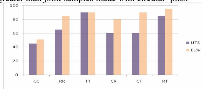
Fig 8. UTS and elongation of joint samples tested with different dual-pin tools.
