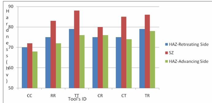
Fig 11. Average hardness values of joint samples in different weld regions in both advancing and retreating sides
