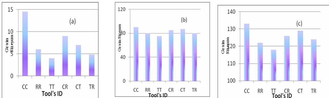
Fig 14. Average grain size for samples welded through use of various dual-pin tools within: (a) SZ, (b) TMAZ, and (c) HAZ.
