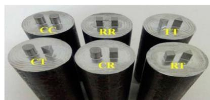
Figure 1. Dual-pin tools with different pin shapes.
