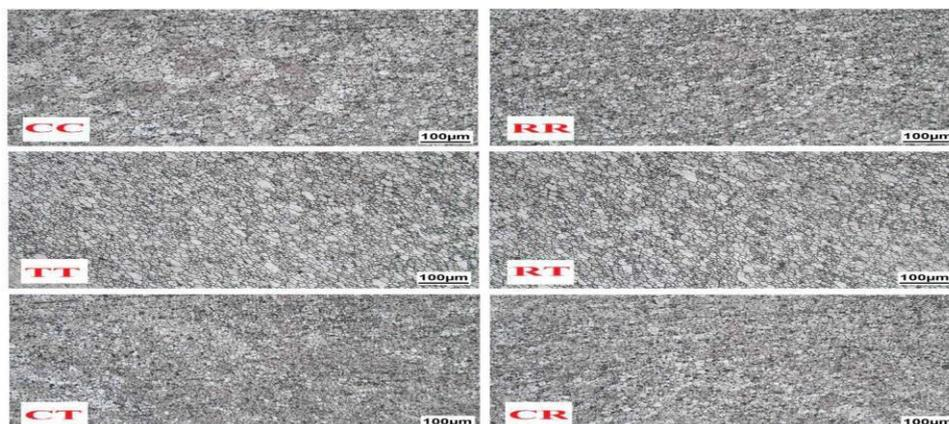
Fig 15. Microstructures of the SZ for joint samples welded by various dual-pin tools.
