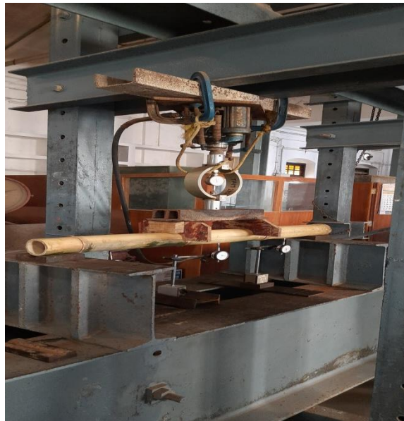
Figure 4. Four-Point Bending Test setup
