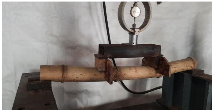
(b) Bending failure at the centre
