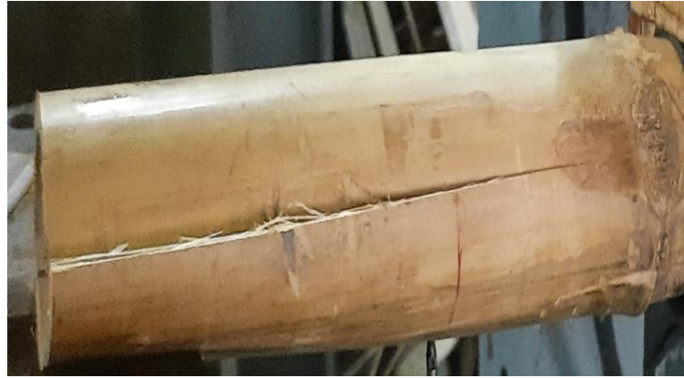
(a) Crushing at the ends of Bamboo Poles
