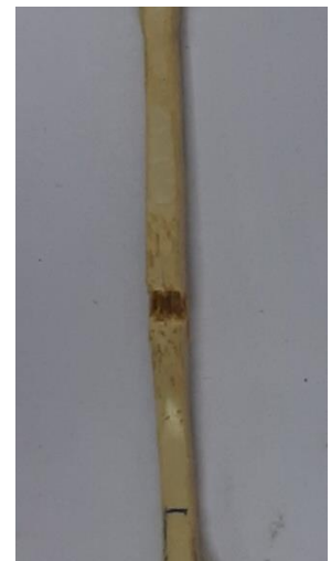
Figure 9. Typical snapping of specimen observed from tensile test
