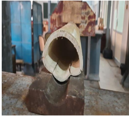
(a) Crushing at the ends of Bamboo Poles
