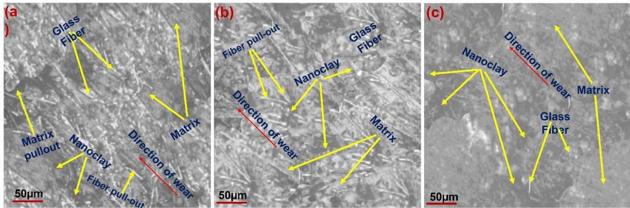
Figure 8. SEM images of fractured surface of (a) UHMWPE/GF/1% Nanoclay
