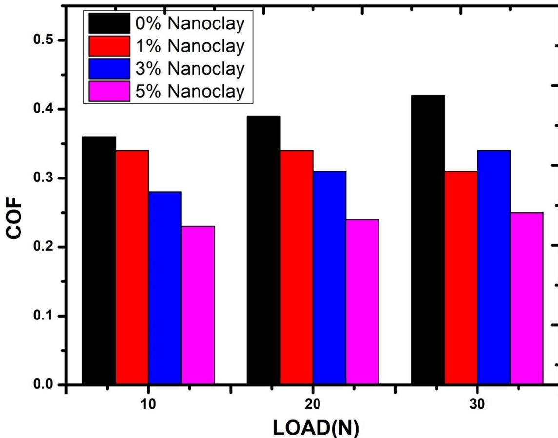
Figure 7. Coefficient of Friction of UHMWPE/GF/X% Nano-clay (X=1%, 3% and 5%)
