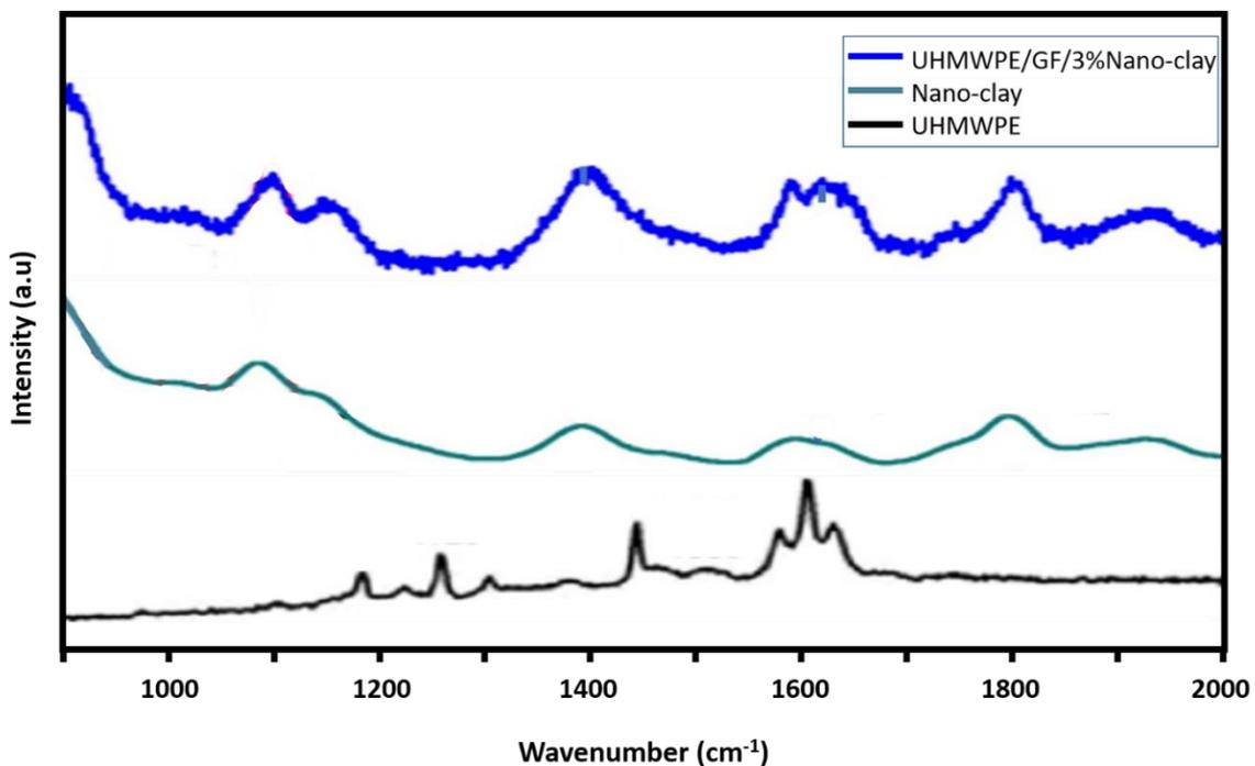
Figure 1. Raman Spectroscopy Evaluation of UHMWPE/GF/3% Nano-clay, Nano-clay and UHMWPE
