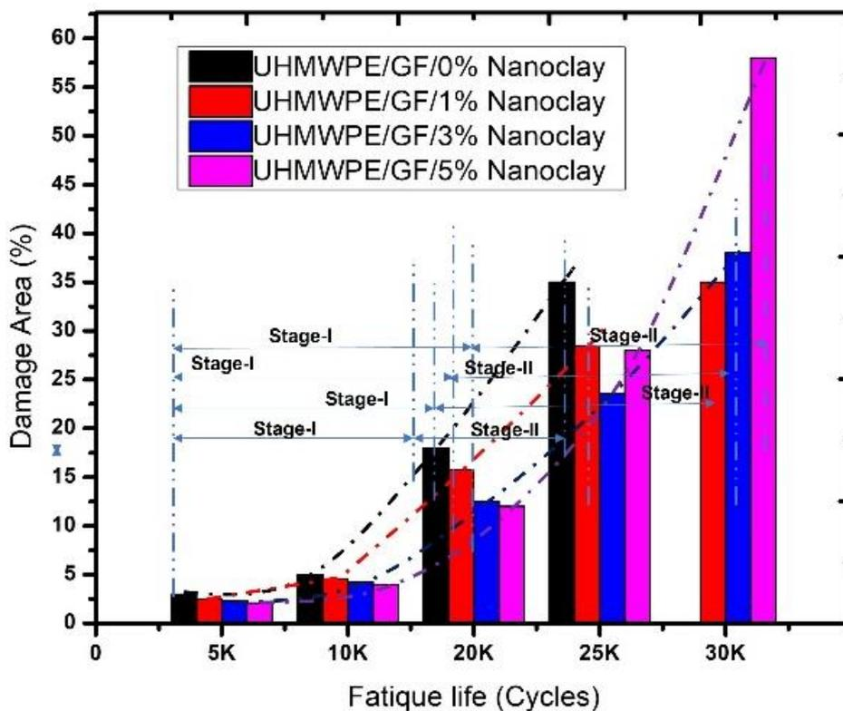
Figure 6. Damaged area divided by total gauge area plotted as a function of fatigue life
