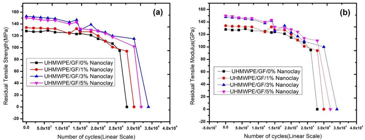
Figure 4. (a) Residual tensile strength and (b) Residual tensile modulus of UHMWPE/GF/Nano-clay hybrid composites.
