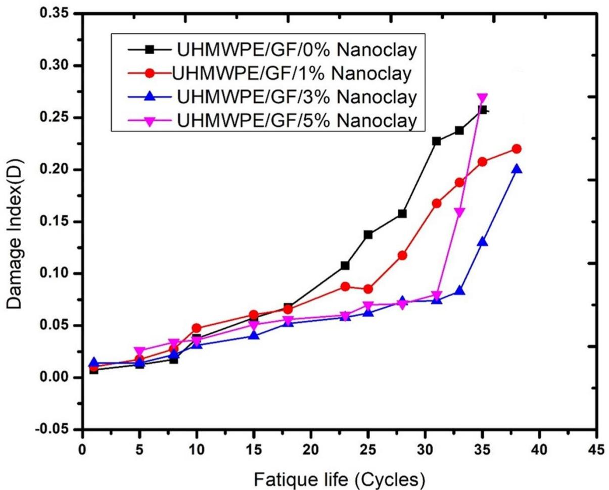
Figure 5. Damage index,  $D$ , plotted a function of fatigue cycles for hybrid composites containing different clay contents
