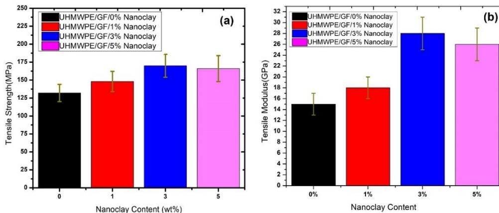
Figure 3. (a) Tensile strength (b) Tensile modulus of UHMWPE/GF/Nano-clay hybrid composites
