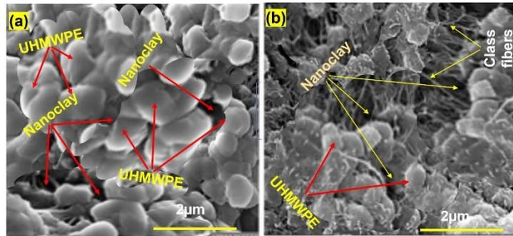
Figure 2. The SEM images of Composite specimens (a) without GFs and (b) with GFs
