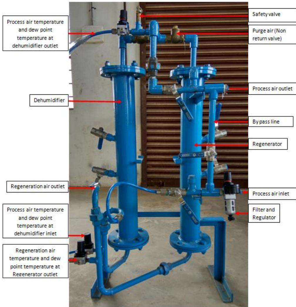
Fig.2 Photographic view of developed setup
