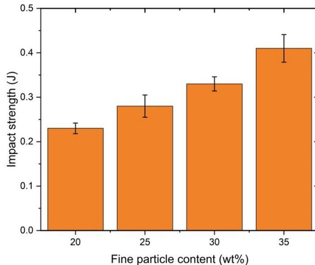
**Figure 3:** Variation in impact strength of fine particle reinforced epoxy composite for varying particle loading
