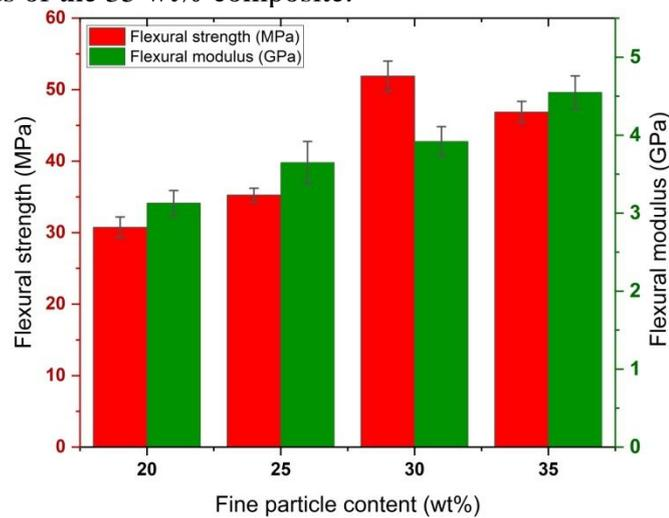
**Figure 2:** Variation in flexural strength and modulus fine particle reinforced epoxy composite for varying particle loading
