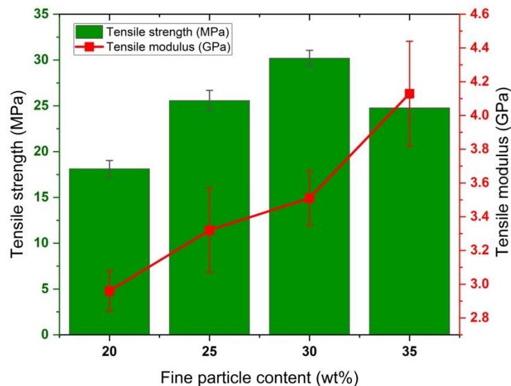
**Figure 1:** Variation in tensile strength and modulus of fine particle/epoxy composites for varying particle loading
