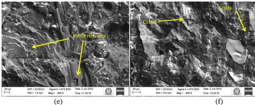
**Figure 4:** SEM images of banana fine particle/epoxy composites: (a) 25 wt% composite after tensile test, (b) 35 wt% composite after tensile test, (c) 25 wt% composite after flexural test, (d) 35 wt% composite after flexural test, (e) 25 wt% composite after impact test, and (f) 35 wt% composite after impact test
