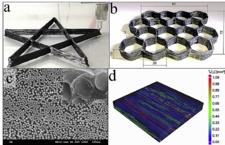
**Figure 7.** Photographs of three dimensionally printed (a) structure of pentagram (b) honey comb based structure (c) SEM micrograph of the cross section of the 3D structure and (d) analysis of interior structure using software as illustrated by Ming et al. [8]
