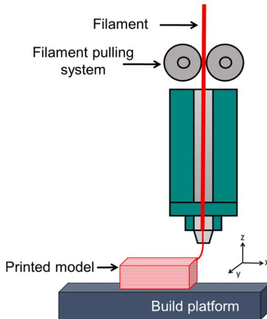
**Figure 1.** Principle of operation of the FDM Process as illustrated by Shanmugam et al. [22]
