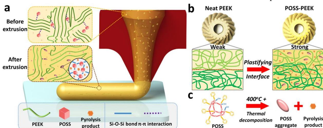
**Figure 5.** Graphical representation of the three dimensionally printed PEEK/POSS nano composite structures (a) morphology based modification induced through POSS during the three dimensional printing (b) POSS based pyrolysis products serves as plasticizers in enhancing the interface relevant binding strength and (c) process of pyrolysis & POSS related products as portrayed by Li et al. [41]
