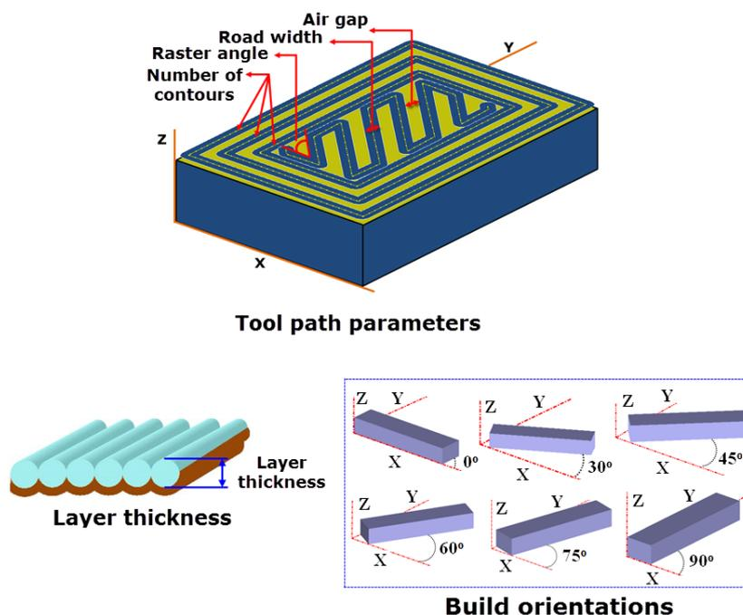
**Figure 2.** Various parameters of the FDM Process as portrayed by Mohamed et al. [29]
