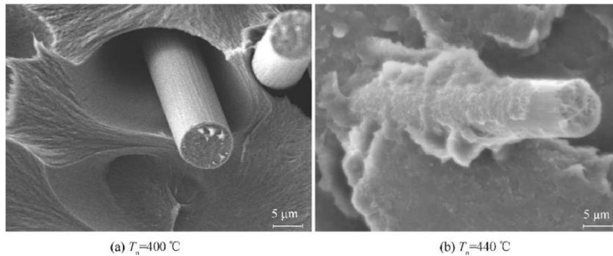
**Figure 6.** SEM micrographs of the interface amidst the PEEK and fiber in the three dimensionally printed composite structures at (a) 4000c and (b) 4400c nozzle temperature as observed by Wang et al. [45]
