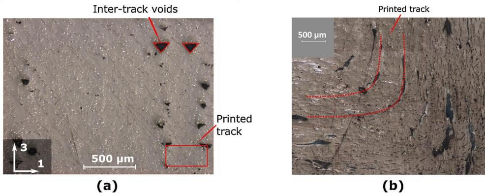
**Figure 3.** Microstructural images of the three dimensionally printed short fiber based nylon revealing its (a) cross section and (b) top view of its corner as described by Blok et al. [33]
