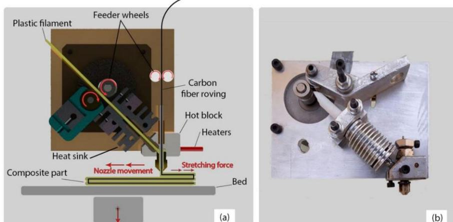
**Figure 4.** (a) Graphical illustration of designed innovative extruder and (b) actual photograph of successfully fabricated extruder as recorded by Heidari-Rarani et al. [34]
