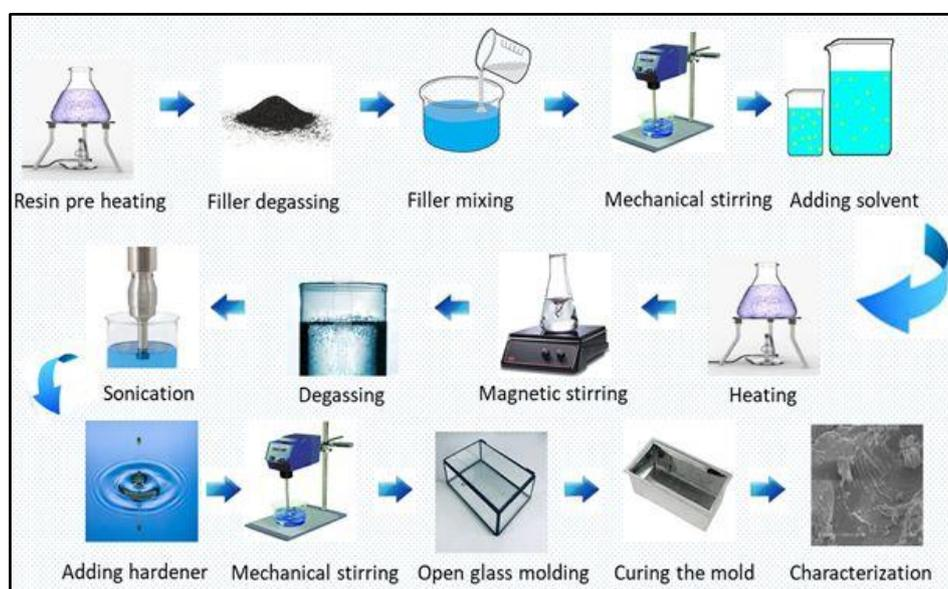
Fig. 1. Graphical process flow chart of making filler reinforced polymer composites
