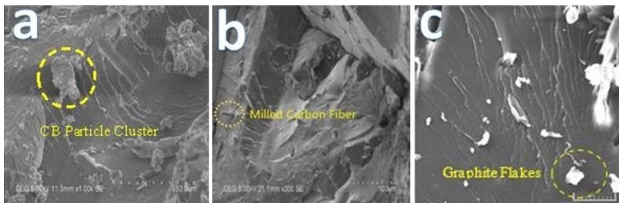
Fig. 2. SEM images of cross section of a) CB/epoxy, b) MCF epoxy, c) NGF epoxy composites
