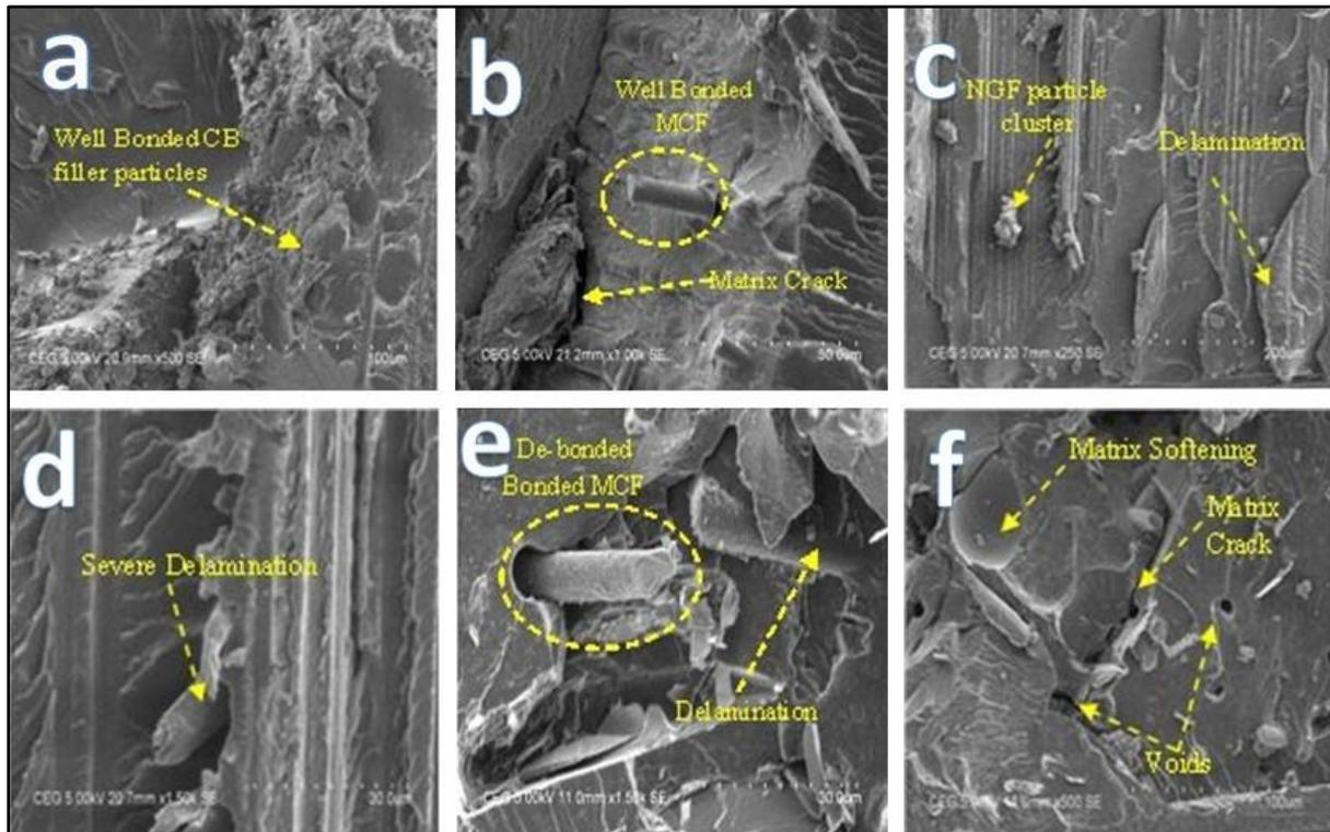
Fig. 8. SEM fracture tensile surface morphology. a) 2wt% CB filler b) 2wt% MCF filler c) 2wt% NGF filler d) 12wt% CB filler e) 12wt% MCF filler f) 12wt% NGF filler
