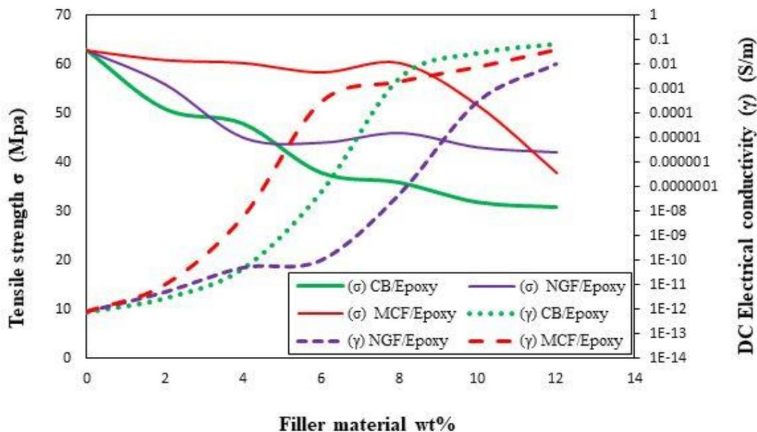
Fig. 10. Evaluation of mechanical and electrical properties of filler/epoxy composites
