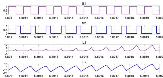
**Fig.11. Inductor currents with switching pulses**
