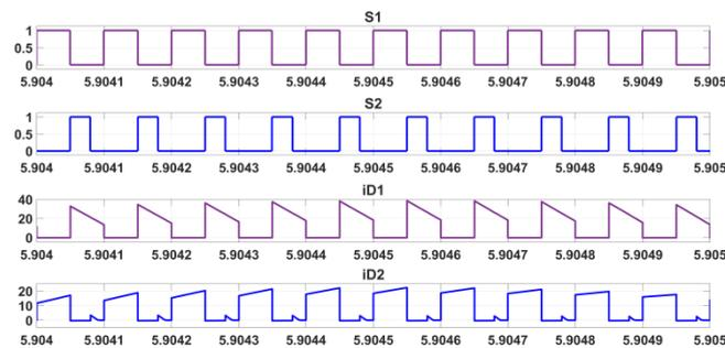
**Fig.10. Diode currents with switching pulses**
