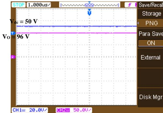
**Fig.13. Output voltage and capacitor voltage waveforms**
