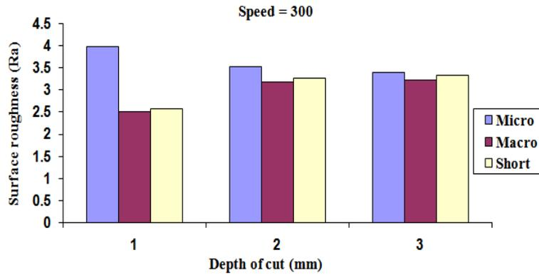
**Figure 6:** Variations of surface roughness based on the depth of cut with a cutting speed of 300 rpm
