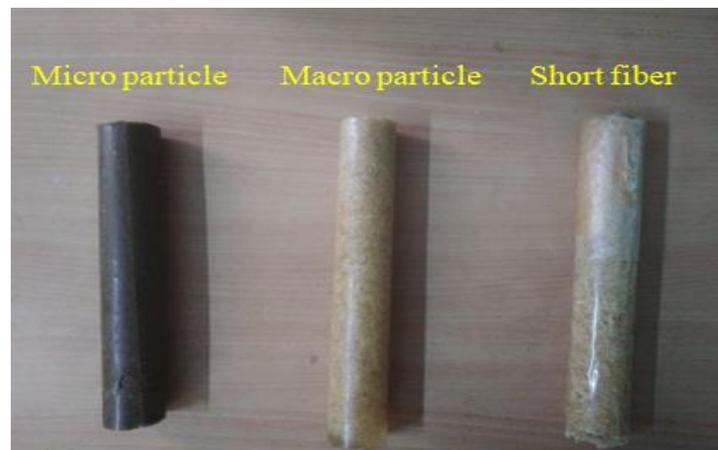
**Figure 1:** Digital image of the composite rod for micro, macro particle and short fiber reinforced with epoxy composites
