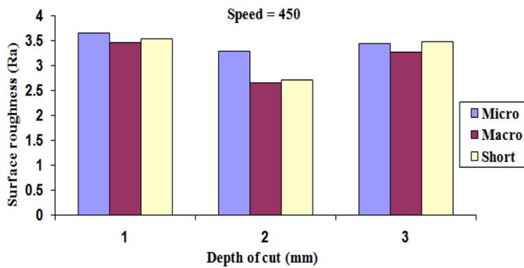
**Figure 7:** Variations of surface roughness based on the depth of cut with a cutting speed of 450 rpm
