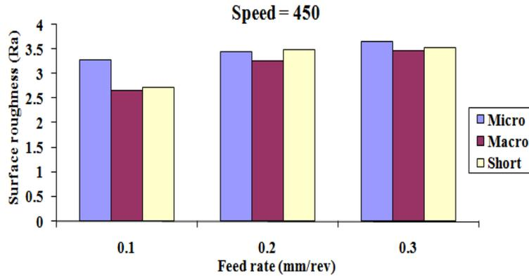
**Figure 4:** Variations of surface roughness based on the feed rate with a cutting speed of 450 rpm
