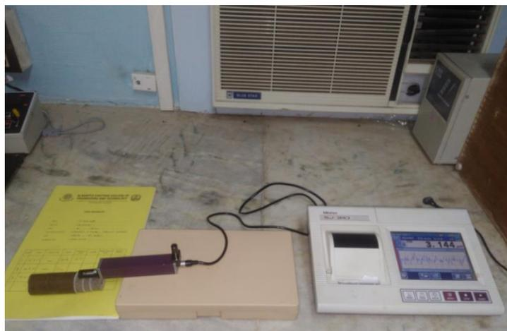
**Figure 2:** Digital image of composite specimen during surface roughness measurement
