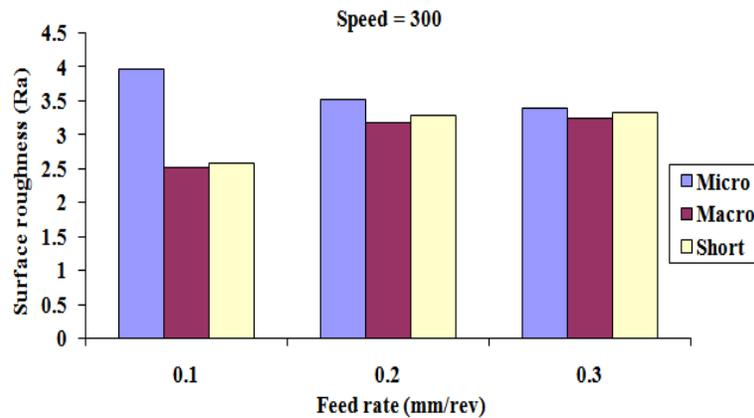
**Figure 3:** Variations of surface roughness based on the feed rate with a cutting speed of 300 rpm
