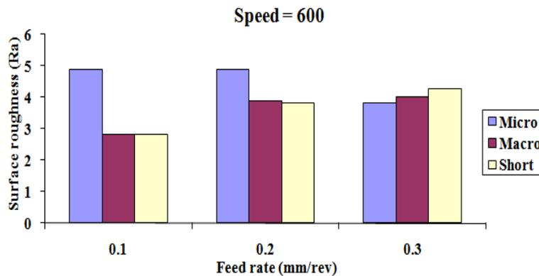
**Figure 5:** Variations of surface roughness based on the feed rate with a cutting speed of 600 rpm
