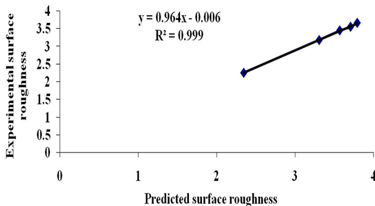
**Figure 13:** Comparison between the experimental and predicted surface roughness during turning of macro particle reinforced epoxy composite
