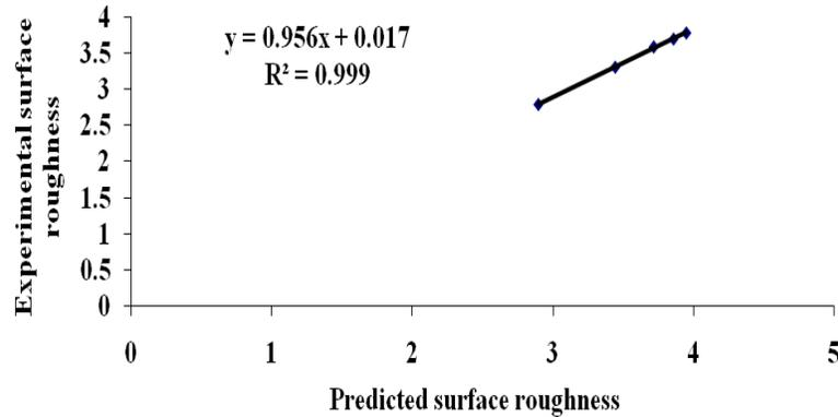
**Figure 14:** Comparison between the experimental and predicted surface roughness during turning of short fiber reinforced epoxy composite
