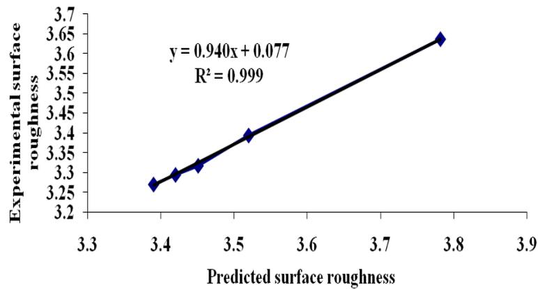
**Figure 12:** Comparison between the experimental and predicted surface roughness during turning of micro particle reinforced epoxy composite
