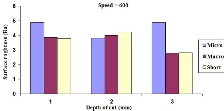
**Figure 8:** Variations of surface roughness based on the depth of cut with a cutting speed of 600 rpm
