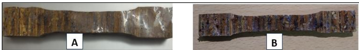
Fig.3 Specimens prepared for UTM testing as per ASTM 3039 Standards A) without Nano-silica B) with the addition of Nano-silica
