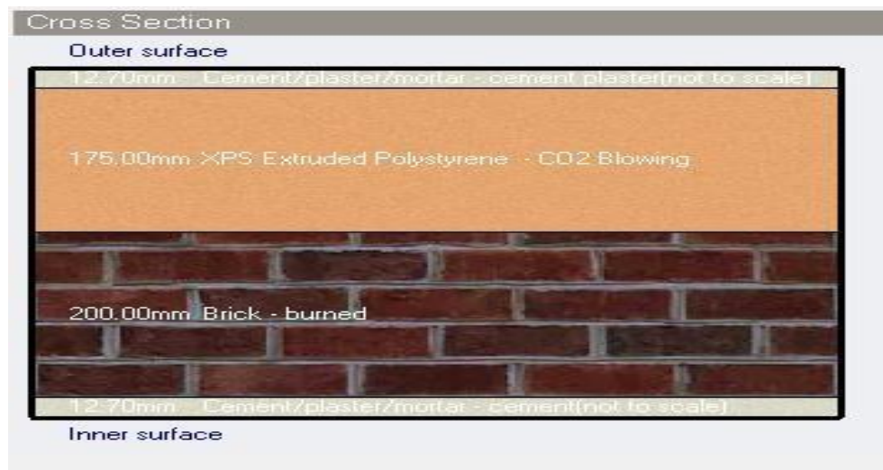
Figure 5 Polystyrene insulated wall material
