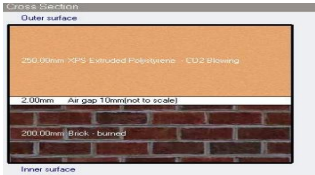
Figure 7 Cavity wall with polystyrene insulation
