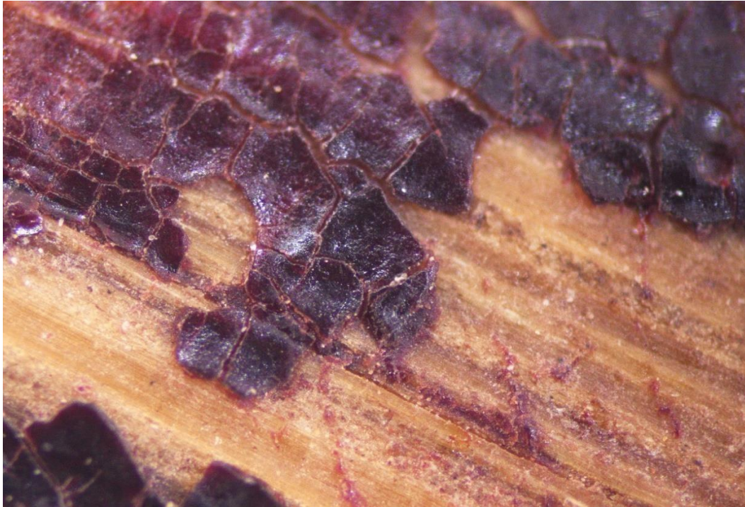
Fig.10: Microcracks inside dry blood stain deposited on dicot wood surface at 40x magnification.
