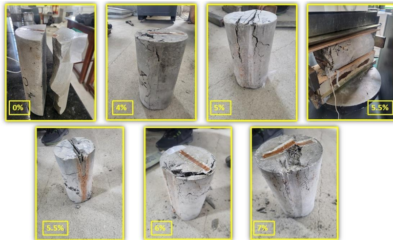
Figure 7: Failure Mechanism of HPSIFCON in Indirect Tension
