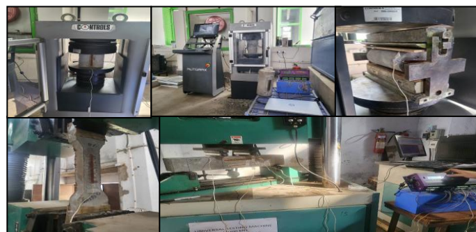
Figure 4: Test setup and instrumentation (top left to bottom right): Compressive test, Modulus of elasticity and Poisson's Ratio, split tensile, direct tensile test and flexural test.
