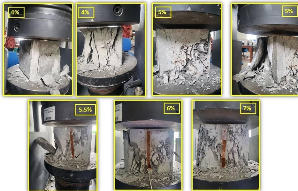
Figure 5: Failure Mechanism of HPSIFCON in Compression
