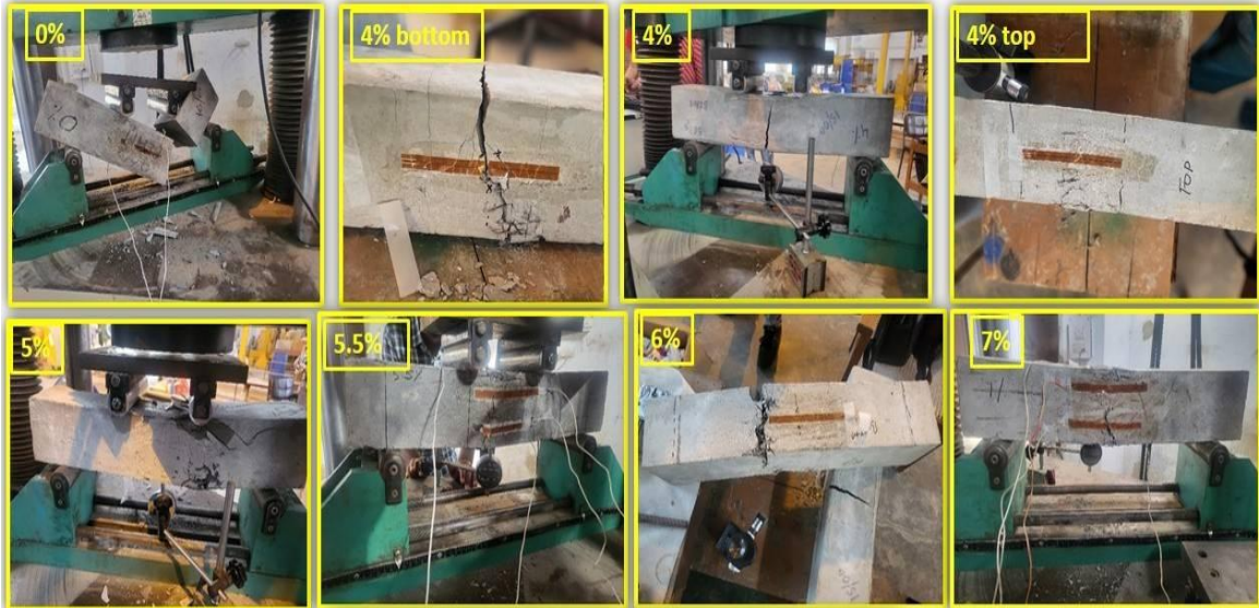
Figure 6: Failure Mechanism of HPSIFCON in Flexure
