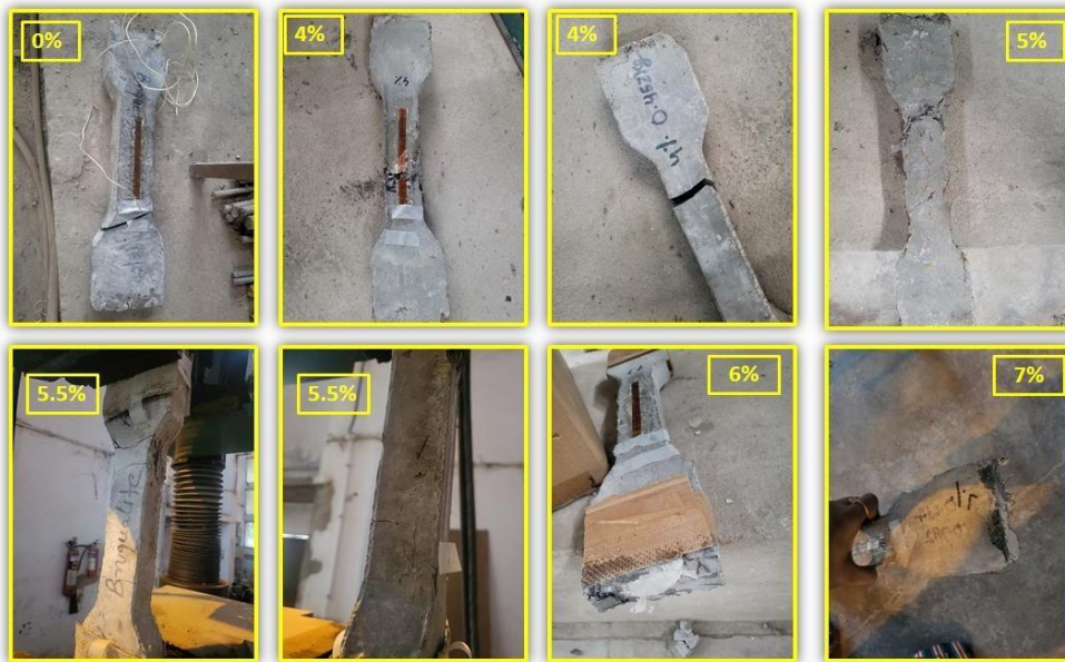
Figure 8: Failure Mechanism of HPSIFCON in Direct Tension
