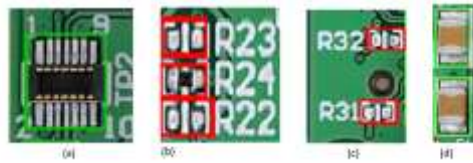
Figure 8: Image of highlighted misaligned components and missing components. (a) & (d) Properly aligned component with green highlighted (b) & (c) Improperly aligned component and missing components.
