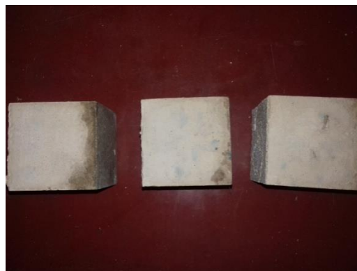
Figure 9: Mortar Cubes after Casting
