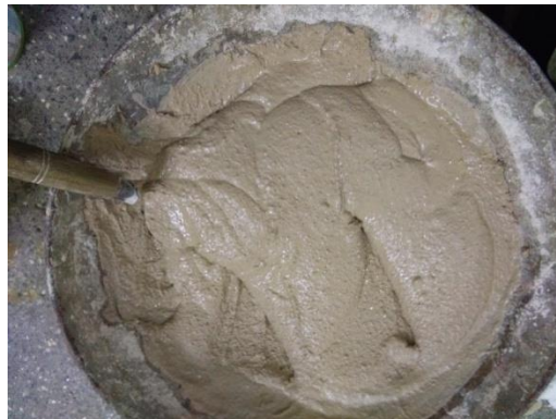
Figure 7: Hand Mixing of Geopolymer Mortar for M40
