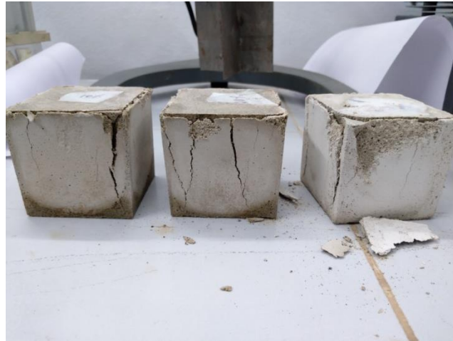
Figure 11: Mortar Cubes after Testing
