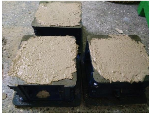
Figure 8: Casting of Geopolymer Mortar
