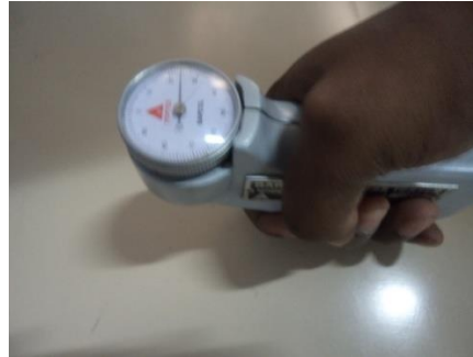
Figure 2 Hardness measured by Barcol hardness tester
