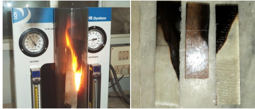
Figure 4 Fire-retardant test and burned composite specimens
