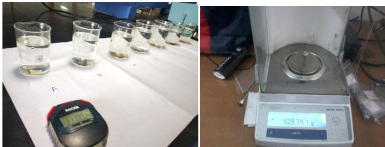
Figure 1 Moisture absorption and weight measurement setup
