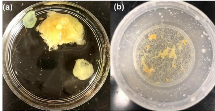
**Fig. 2.** Dispersed electrospun PFS inside the precursor gel
