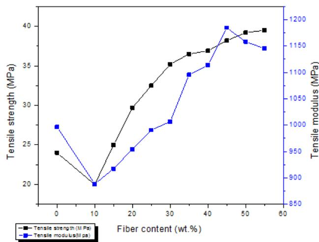
**Fig. 4.** Mechanical properties of ceramic-0.5 wt% PEO fiber
