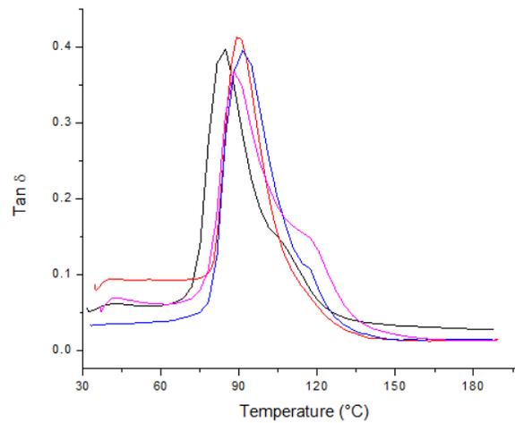
**Fig. 6.** Dynamic Mechanically oriented properties 0.5 wt% of PEO fiber composite
