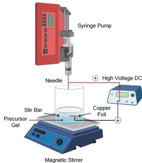
**Fig. 1.** The experimental setup of wet Electrospun PEO fiber-ceramic composite synthesis
