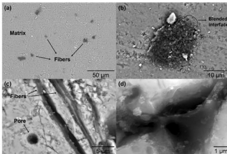
**Fig. 3.** Microstructure of the tough surfaced ceramic
