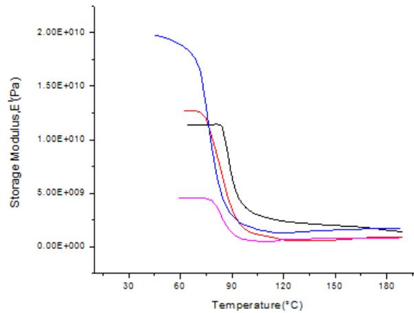
**Fig. 5.** Fluctuation of E1 of plain epoxy and nanocomposite as a function of temperature
