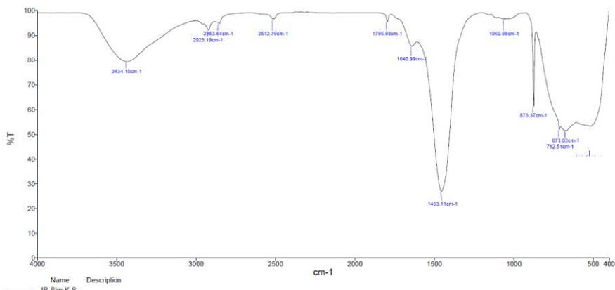
Fig. 1. FTIR analysis of the nano catalyst
