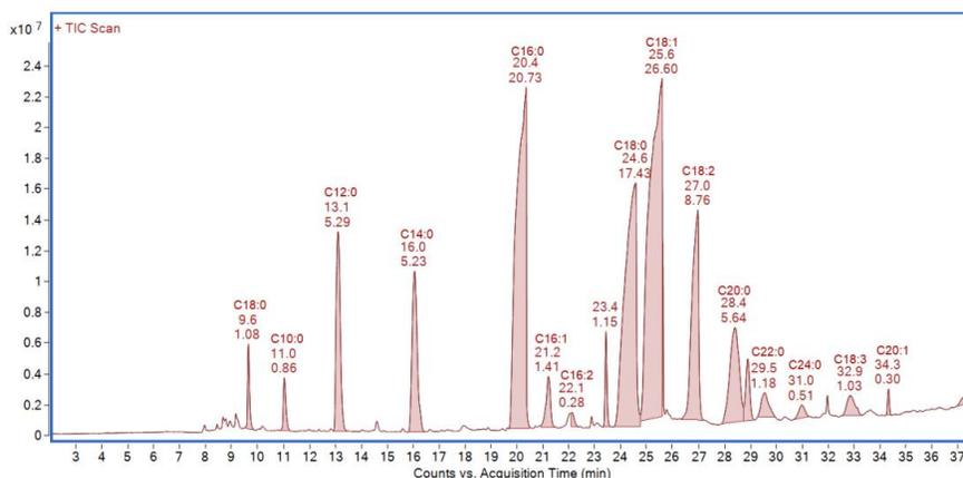
Fig. 7. GC-MS analysis of the biodiesel produced from *Ceiba penandra* oil
