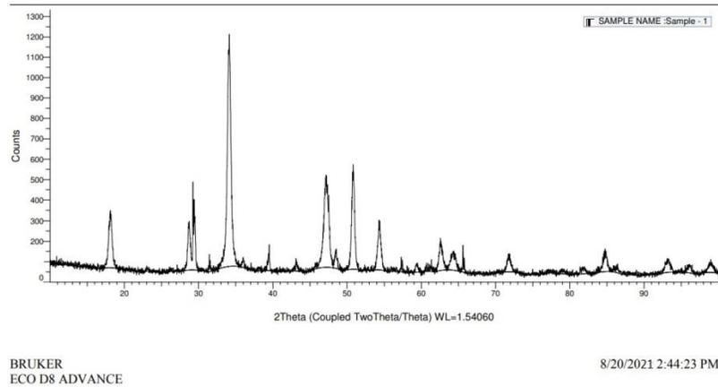
Fig. 2. XRD analysis curve of the nano catalyst
