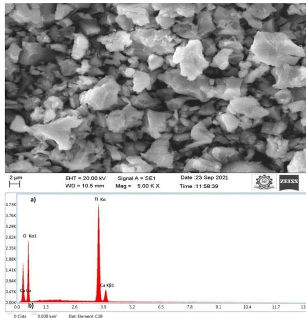
Fig. 3. SEM images of the nano catalyst at magnifications a) 50 KX and b) c) corresponding EDX graph.
