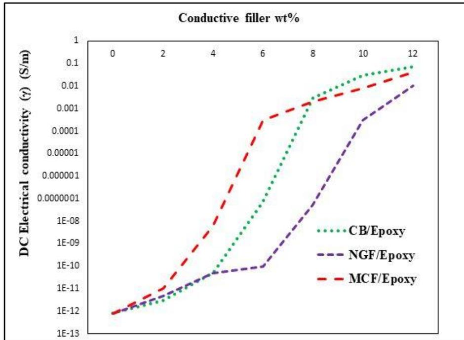
Fig. 9. DC electrical conductivity of filler reinforced epoxy composites
