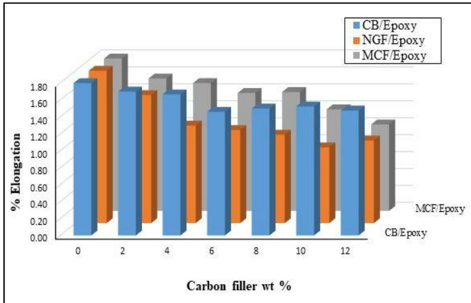
Fig. 7. Percentage elongation of carbon filler/epoxy composites
