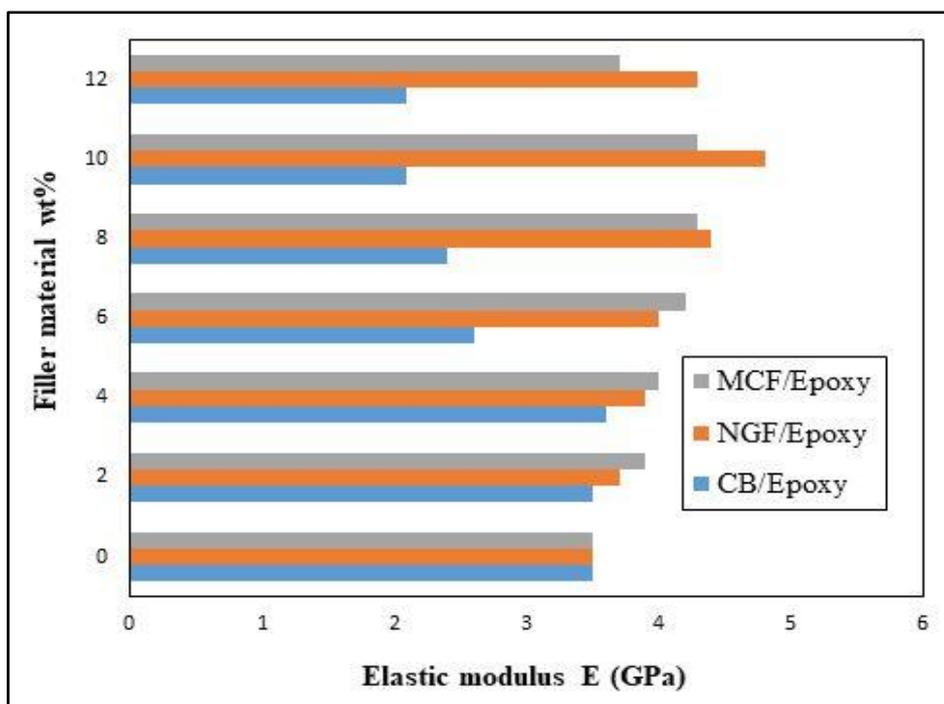
Fig. 6. Elastic modulus of filler /epoxy composites
