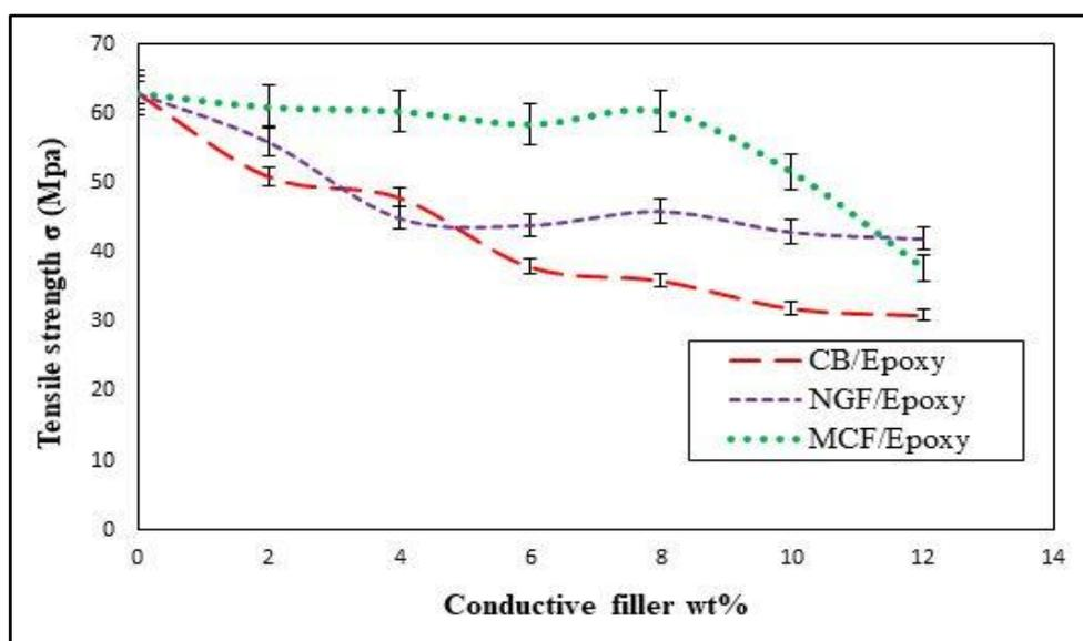
Fig. 5. Tensile strength of filler reinforced epoxy composites
