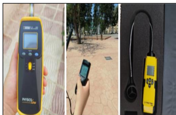
Figure 9: The hygrometer thermometer Chauvin Arnoux, in the centre: Handheld thermo-hygrometer HANNA, on the right: A propeller anemometer TROTEC ba16. (Source: Author 2022.)
